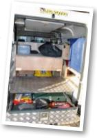
A full-height second bulkhead now splits the cab from the load area, preventing any larger items from embedding themselves in the back of our heads in the event of a crash. This also improves security for all of the kit in the back of the truck, while making the cab a little less claustrophobic.
